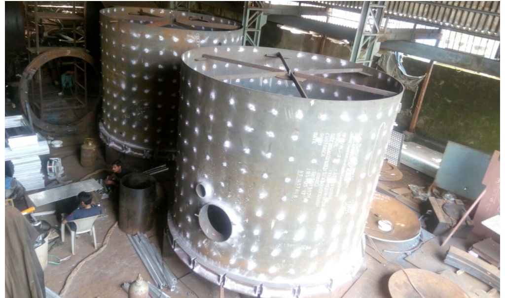
Skirt with Nuts welded for insulation support. Welding with DP test. Made for Godrej & Boyce
