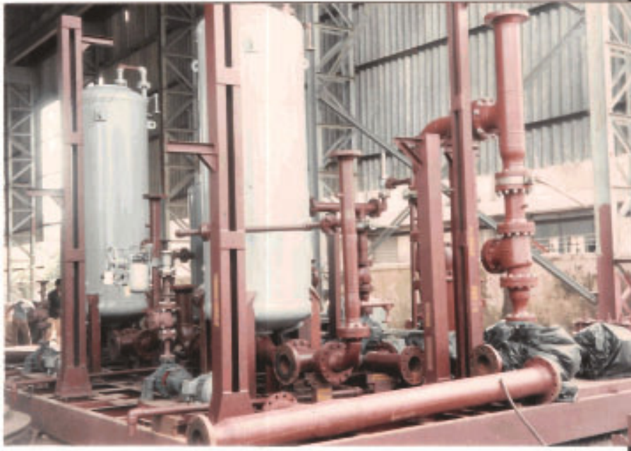
Skid with pumps, motors and instrumentation. Made for ION Exchange India.
